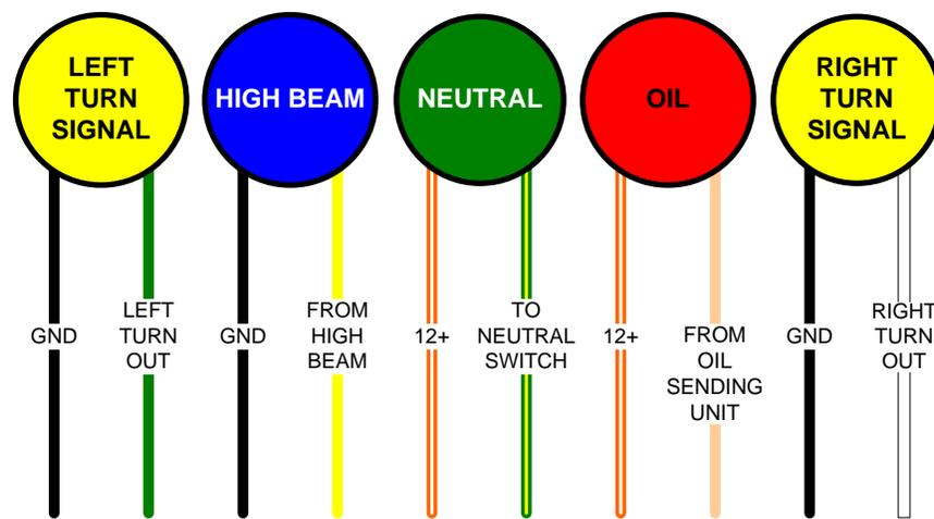
When wiring the indicator lights, be sure to twist ALL (3) of the black wires together and BOTH (2) of the orange/white wires together when attaching to our harness.
