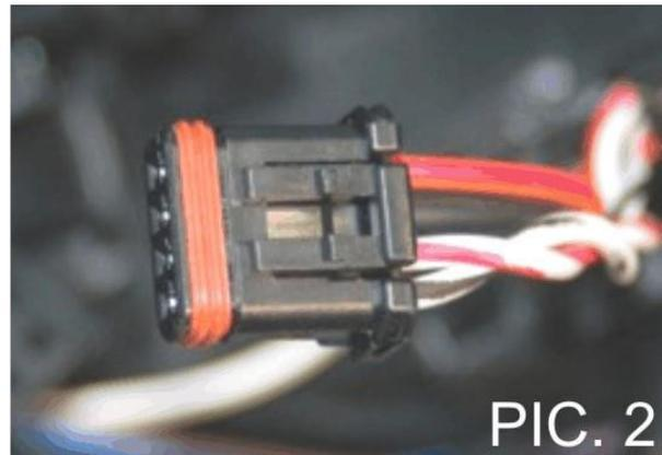
Connect the 4-position female connector of the NCBC-N01 to the **RIGHT SIDE** 4-position male connector (PIC 1) under the fuel tank. **This harness may not be extended and it is mandatory to use this unmodified connection for proper voltage supply of the NCBC-N01.** The left plug may be left without any connection and should be protected against moisture using electrical tape or heat shrink.
